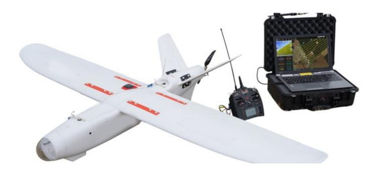
The UAVi X-200 High Wing UAV is an easy-to-launch, terrain mapping and operational surveillance. It offers superb stability, silent and fast cruise flight and tons of Power with its dual motor configuration. With bigger space in its belly, UAVi X-200 offers to carry 16,000 mah batteries and can offer flight times up to 60 minutes depending on weather conditions.
